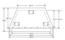
\**Note:* 14 <sup>1</sup>/<sub>4</sub>" is total firebox cavity depth including brick liner. 13 <sup>1</sup>/<sub>4</sub>" is depth of flat floor including brick liner.
